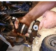
**6.** Remove the LH upper bearing carrier bolt from the upper A-Arm.
