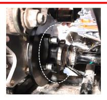
**9.** Remove the (2) 8mm hex bolts and upper 15mm bolt that secure the gear case upper mount to the frame and remove it.
