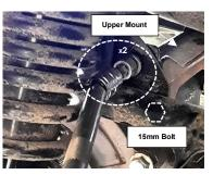
**10.** Remove the lower 15mm bolts attaching the gear case to the frame, then remove it from rear of the vehicle.
