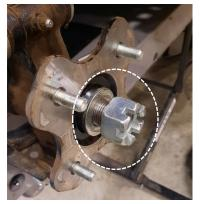
5. Remove the RH upper bearing carrier bolt from the A-Arm. Tilt the carrier downward and remove the RH CV shaft from the carrier, then pull sharply to remove it from the rear gear case.
